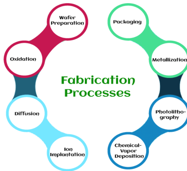
Fig 1.3: Process Flow of IC Fabrication
